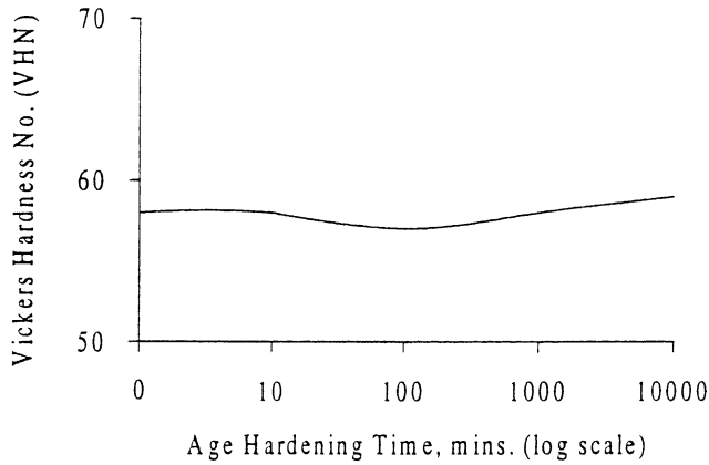
Fig. 8. Vickers hardness vs age hardening time (min) for Al-2.5Mg-0.15Sc alloy.
