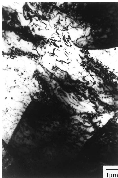
Fig. 3. TEM micrograph of Al-2.5Mg-0.3Sc alloy showing a high dislocation density at the subgrain boundaries.
