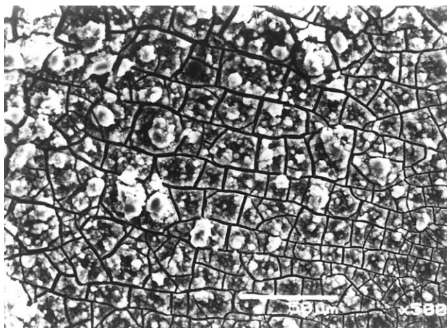
Fig. 15. Photomicrograph of Al-2.5Mg-0.3Sc showing mud cracking (100 \times ).
