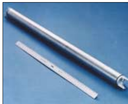
Fig. 3 — An Al-Al 2 O 3 extruded driveshaft reduces weight and enables higher critical speeds.
