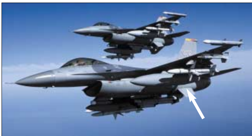
Fig. 1 — The U.S. Air Force F-16 jet fighter includes silicon carbide particulate-reinforced aluminum MMCs in the ventral fin and the fuel access door covers. The arrow indicates the aluminum composite ventral fin.
