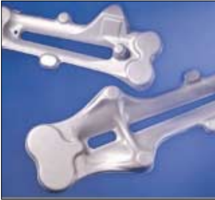
Fig. 2 —Forged 2009/SiC/15p helicopter blade sleeves are used in the Eurocopter.
