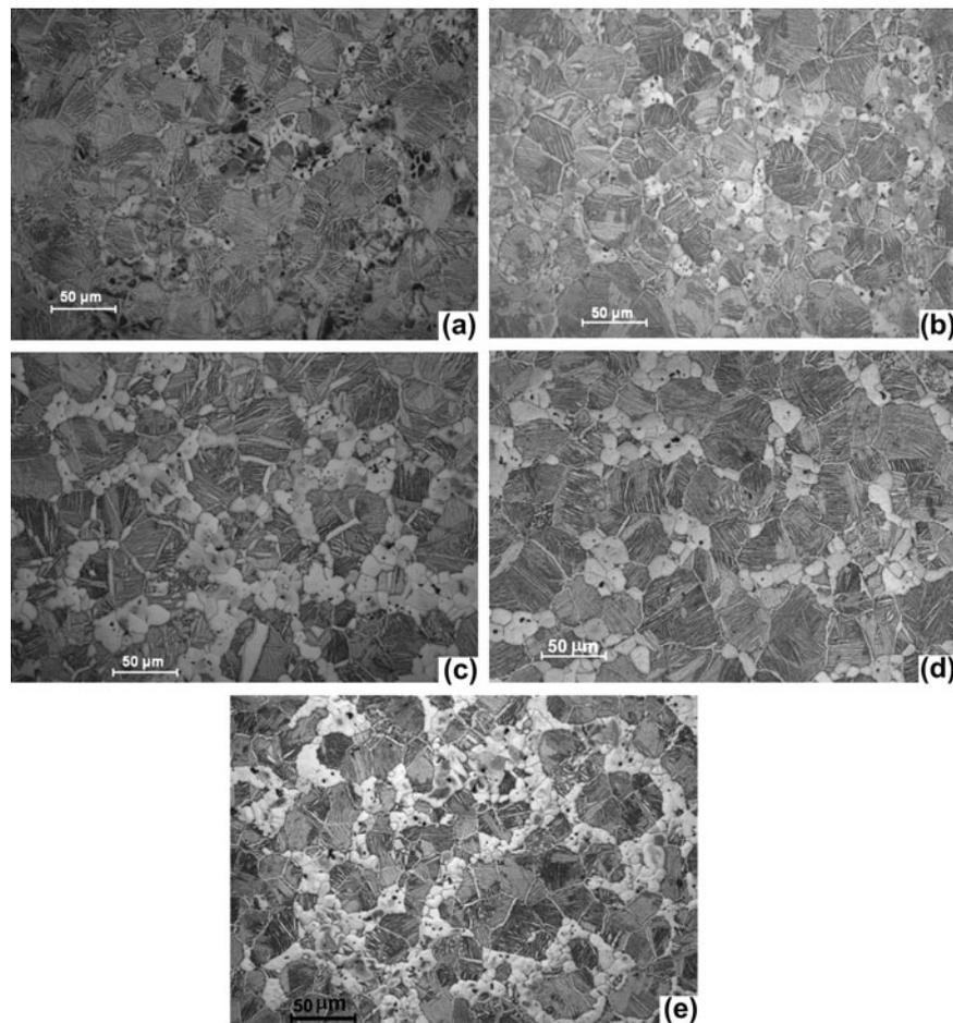
FIG. 3. Optical micrographs of etched cross sections of Ti-6Al-4V densified from BE powders at 10 MPa under thermal cycling conditions (860–1020 °C) for 106 min and subsequently homogenized at 1020 °C for (a) 2 h, (b) 4 h, (c) 16 h, (d), and 64 h (e). As previously described, but sample initially densified at 10 MPa under isothermal conditions (1020 °C) for 110 min and homogenized for 4 h.
