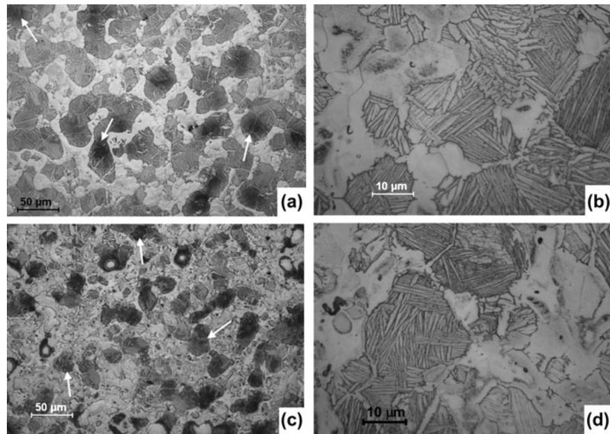
FIG. 2. Optical micrographs of etched cross-sections of Ti-6Al-4V densified from blended elemental (BE) powders at 10 MPa under (a, b) thermal cycling conditions (860–1020 °C) for 106 min and (c, d) isothermal conditions (1020 °C) for 110 min, respectively. Arrows indicate regions of incompletely dissolved Al-40V.
