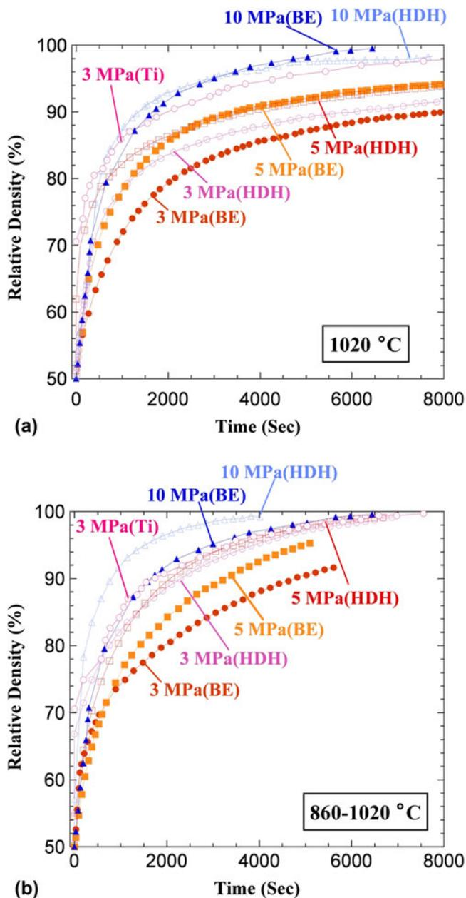
FIG. 4. Densification curves for BE Ti-6Al-4V powders at 3, 5, and 10 MPa (a) isothermally at 1020 °C and (b) under thermal cycling (860–1020 °C). Published densification curves for prealloyed CP-Ti<sup>14</sup> and for prealloyed hydrogenation/dehydrogenation Ti-6Al-4V<sup>7</sup> are also given for comparison.
