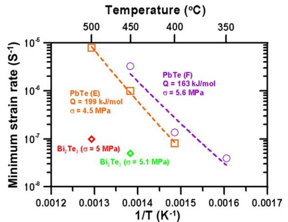
**Fig. 3.** Arrhenius plot of minimum creep rate vs. reciprocal temperature for PbTe, sample E (4.5 MPa) and F (5.6 MPa), showing best-fit creep activation energies. Data for coarse-grained Bi<sub>2</sub>Te<sub>3</sub> at 400 °C are shown for comparison [21].
