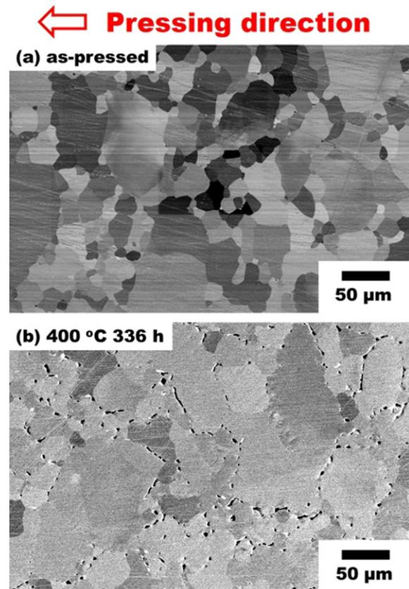
Fig. 1. Secondary ion micrograph of polished cross-section of hot-pressed PbTe (a) before annealing (unetched) and (b) after annealing at 400 °C for 336 h (pores created by 68 wt% HNO<sub>3</sub> etchant).
