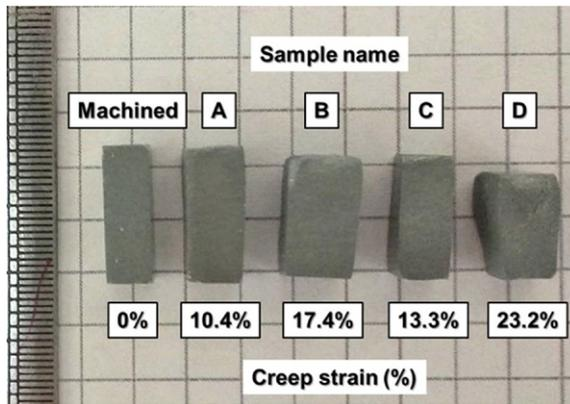
**Fig. 4.** Photographs of PbTe specimen before deformation and specimens A–D after creep deformation at 400 °C.
