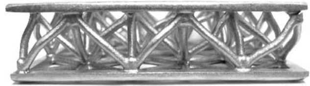
Fig. 9—Photograph of panel B with thick struts deformed under compression.
