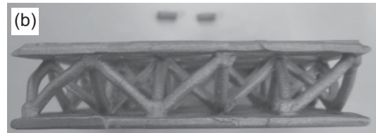
Fig. 5. (a) Compressive stress-strain curves for a Ti-6242 LBS panel and Ti-64 LBS panel, [8] both with same relative density of 16.0%, tested at ambient temperature. (b) Photograph of deformed Ti-6242 panel under room temperature compression.
