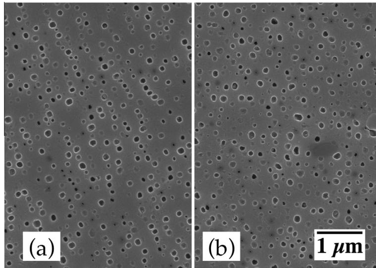
**Fig. 3.** SEM micrograph of etched  $\gamma/\gamma'$  microstructure of Ni–20Cr–3Ti–1Al woven structure, (a) center of a wire and (b) neck between wires. The sample was aluminotitanized at 1000 °C for 1 h, TLP-bonded at 1120 °C for 1 h, homogenized at 1100 °C for 24 h, solutionized at 1200 °C for 2 h, and aged at 900 °C for 12 h.
