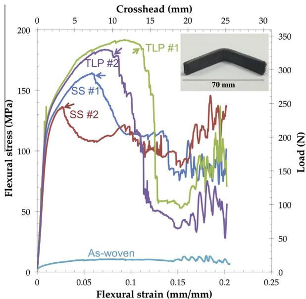
**Fig. 4.** Three-point bending stress–strain curves of Ni–20Cr–3Ti–1Al woven structures after solid-state (SS) bonding or transient-liquid phase (TLP) bonding and aging at 900 °C for 12 h to create a  $\gamma/\gamma'$  microstructure. Numbers 1 and 2 refer to repeat samples. For comparison, a curve for the Ni–20Cr weave is also shown (as woven: unalloyed and unbonded). Inset – deformed TLP-bonded sample.
