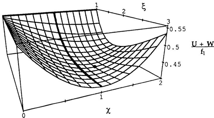
Fig. 2: Graph for  $(U+W)/f_1$  as a function of the relative punching distance  $\xi$  and the relaxation parameter  $\chi$ . A dot marks the location of the minimum,  $(\xi_0, \chi_0)$  and the curve for  $\chi=1$  is highlighted. Mismatching SiC spheroid of aspect ratio 3 in a titanium matrix with  $\Delta T=-300$  K.
