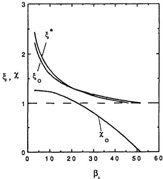
Fig. 3: Punching distance for the system Ti/SiC according to the original model of Ref. (1),  $\xi^*$ , and to the modified model,  $\xi_0$ , as well as punching parameter,  $\chi_0$ , as a function of the spheroid aspect ratio  $\beta_1$ .
