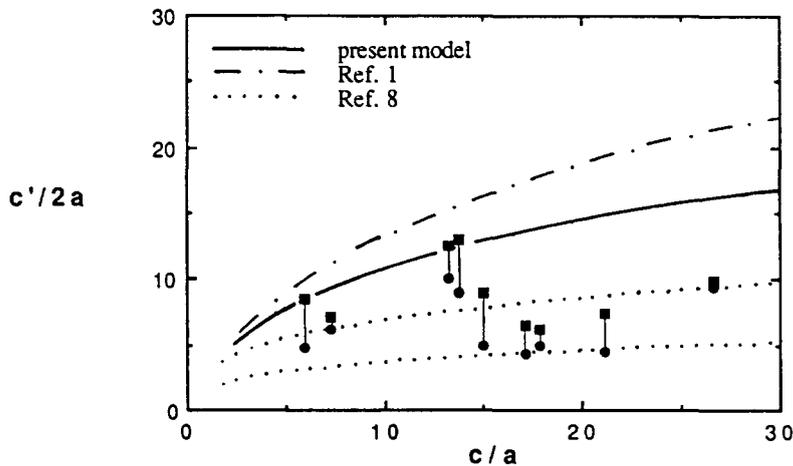
Fig. 5: Punching distance for Taya and Mori's original and modified models assuming no radial mismatch, Eq. [8]. Experimental data points for the system AgCl/glass from Ref. (5).
