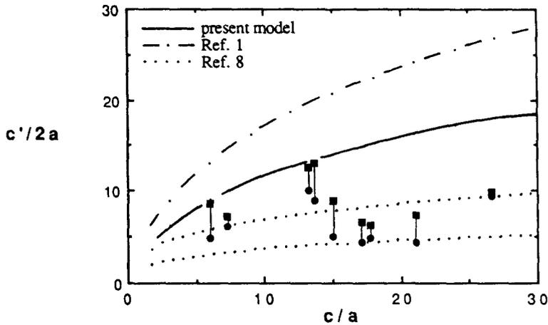
Fig. 4: Dimensionless punching distance for three models and experimental data points from Ref. (5) for the system AgCl/glass.
