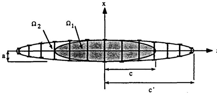
Fig. 1: Spheroidal fiber surrounded by a spheroidal plastic zone of punched prismatic loops (after Ref. 1).
