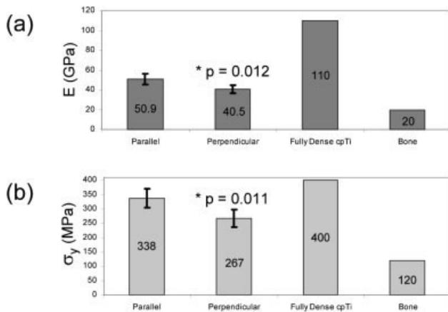
**Figure 4.** Elastic modulus (a) and yield stress (b) measured on 12% porous anisotropic titanium foam created by thermal cycling. Compressive measurements were performed at room temperature with loading direction either parallel or perpendicular to the long axis of the pores. The  $p$  values are for a 95% confidence interval.
