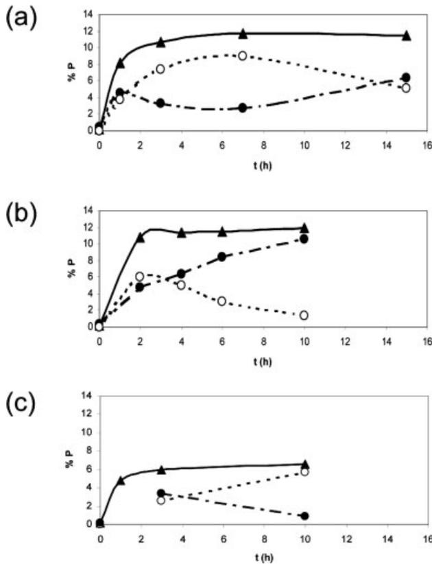
**Figure 2.** Plots of porosity *versus* time for foams created by thermal-cycling (830–980°C) (a); high-temperature isothermal treatment at 1250°C (b); and low-temperature isothermal treatment at 903°C (c), corresponding to the effective temperature of the thermal cycles. Plots show the temporal evolution of total porosity (▲), open porosity (○), and closed porosity (●).
