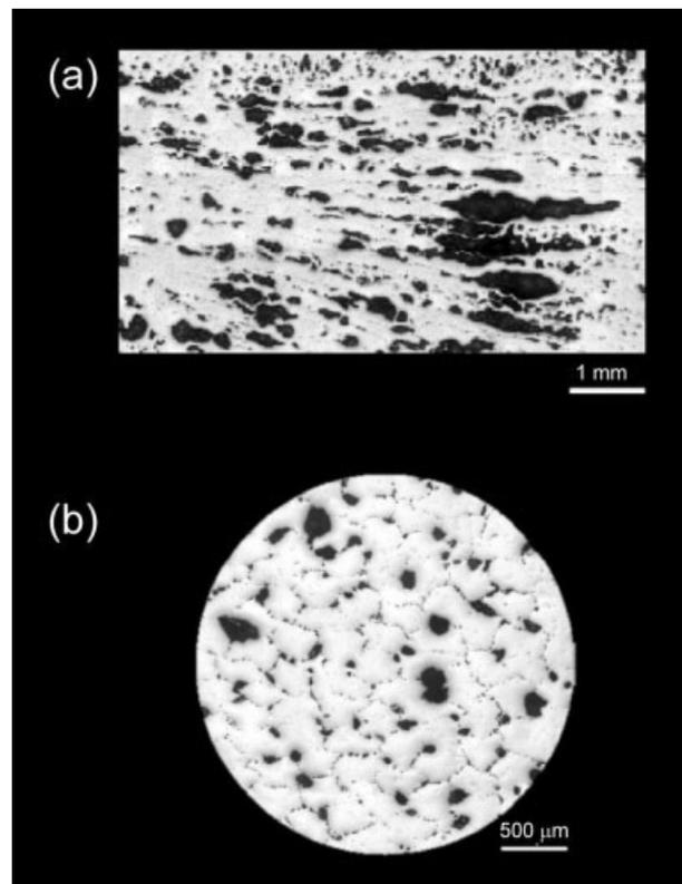
**Figure 3.** Longitudinal (a) and transverse (b) optical micrographs of 12% porous anisotropic titanium foam created by thermal cycling. Both large, elongated, aligned pores and small, equiaxed pores are visible.
