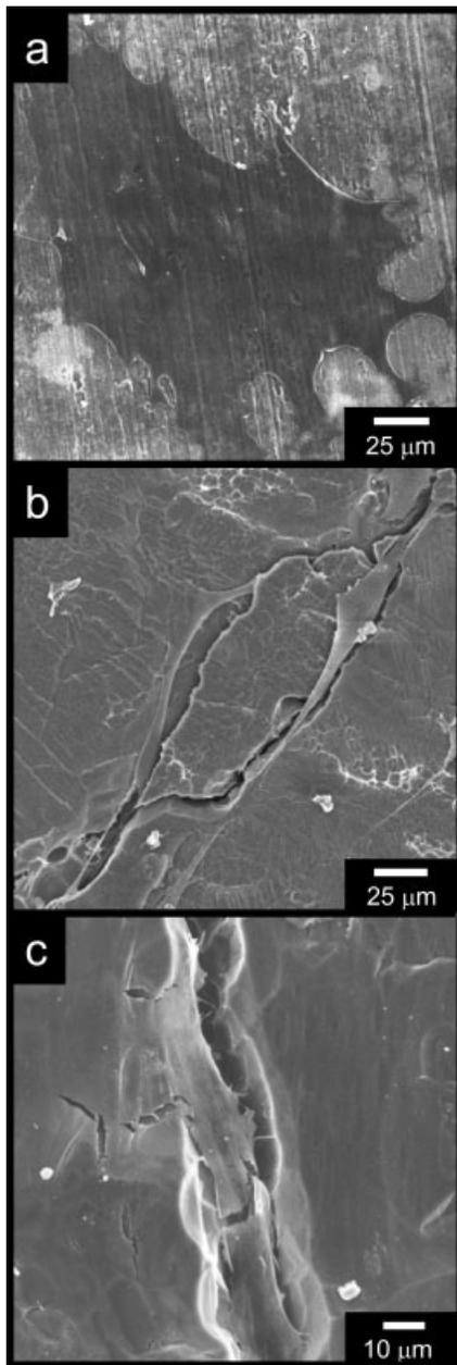
**Figure 7.** Scanning electron micrographs of primary rat osteoblasts growing on a flat titanium surface (a) and along elongated pores (b and c) of titanium with 12% anisotropic pores. The cell on the flat titanium surface has adopted a typically flat, spread morphology, while cells on pores are seen extending along and climbing down into pores.
