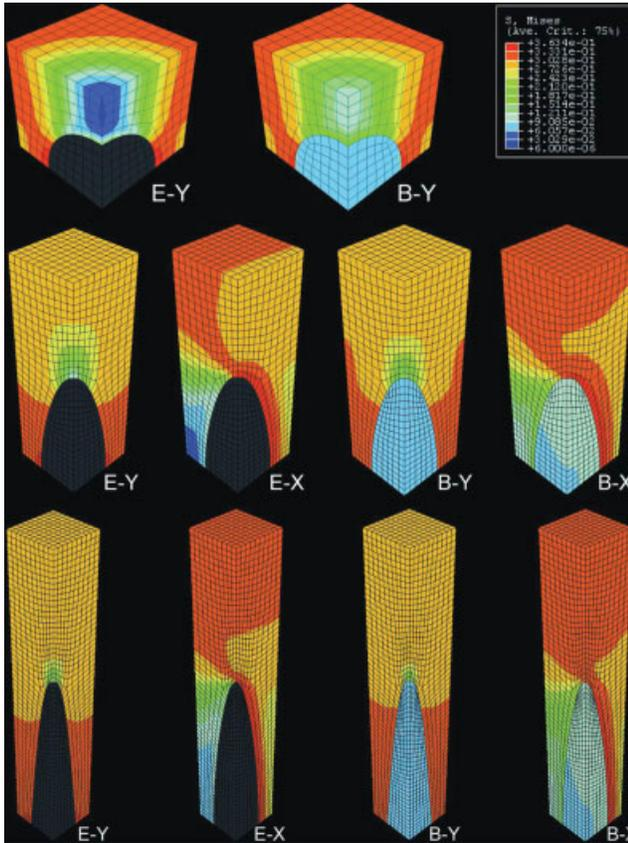
**Figure 6.** Maps of von Mises equivalent stresses in 12% porous titanium containing pores of aspect ratios 1, 3, and 6 (top, middle, and bottom, respectively) Maps are labeled according to their contents (E, empty; B, bone-filled) and the direction of loading with respect to the long axis of the pores (Y, longitudinally; X, transversely).
