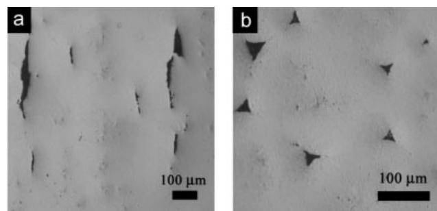
**Figure 1.** Longitudinal (a) and transverse (b) optical micrographs of hot isostatically pressed wire billet prior to foaming, showing large, elongated pores in the space between the wires.
