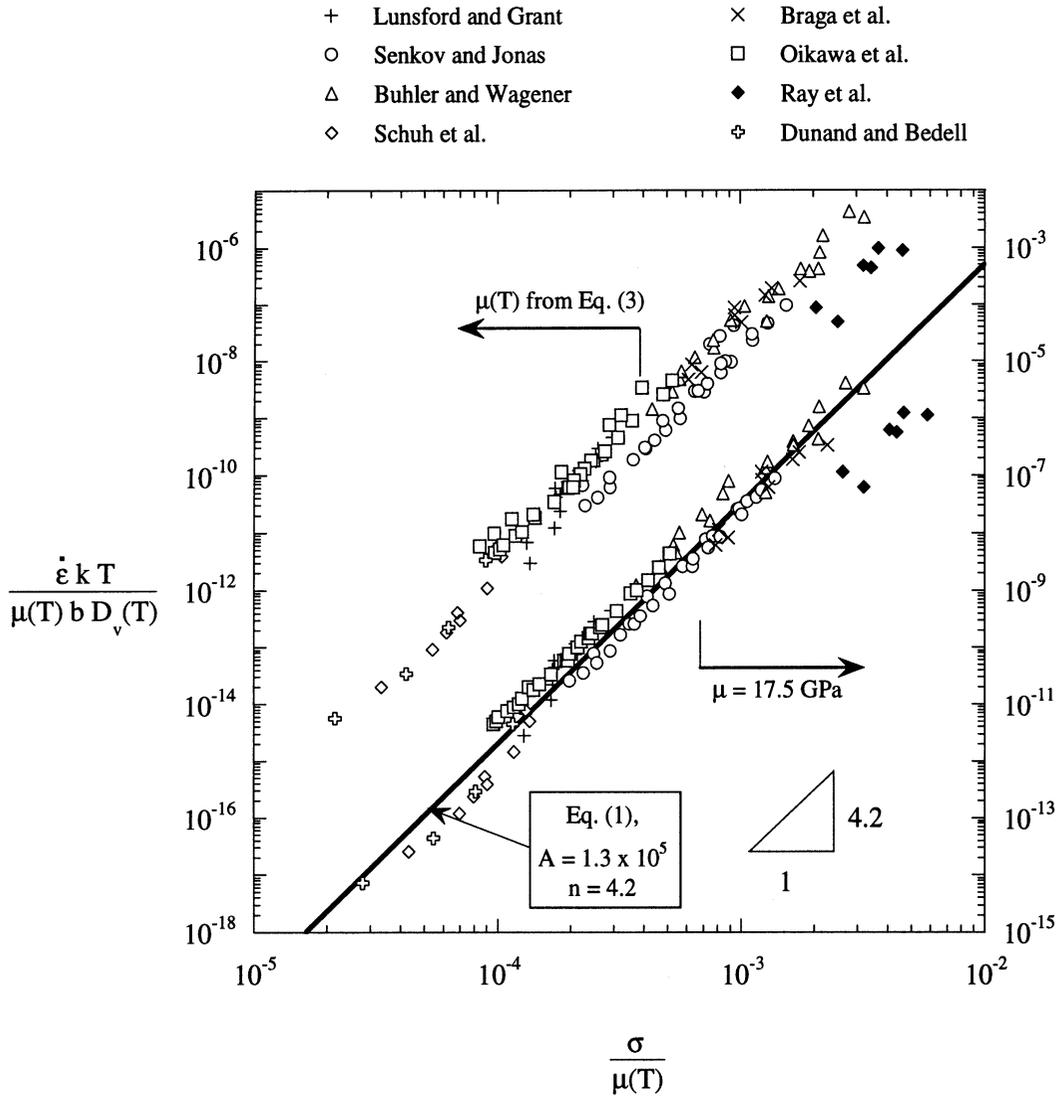
Fig. 2. Temperature-compensated creep rate vs. modulus-compensated stress, for the data sets shown in Fig. 1. Upper data set uses the shear modulus of Eq. (3), and lower set uses a temperature-independent modulus. Best fit excludes data of Ray et al. [7].
