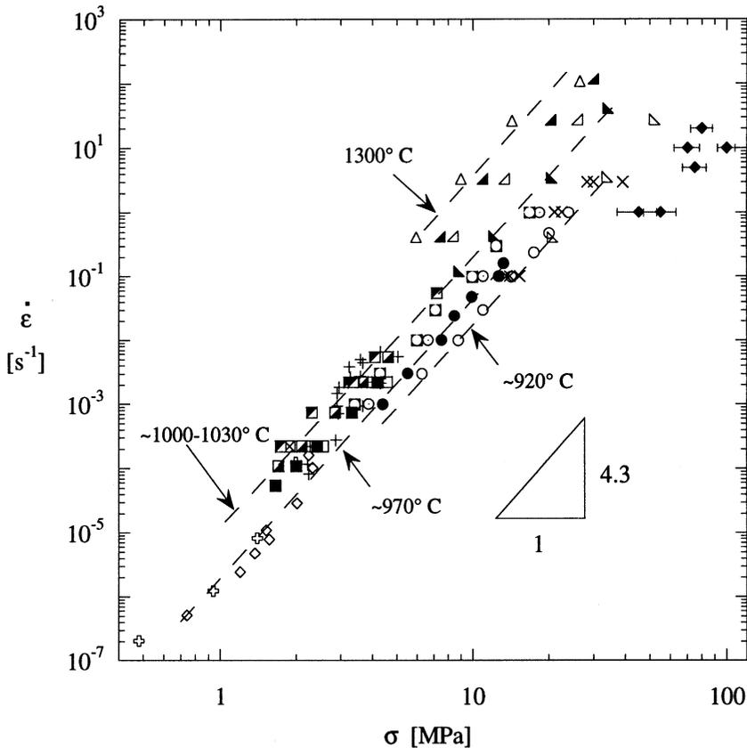
Fig. 1. Creep rate of  $\beta$ -Ti as a function of applied stress. Dashed lines show approximate temperatures for the nearby data points.
