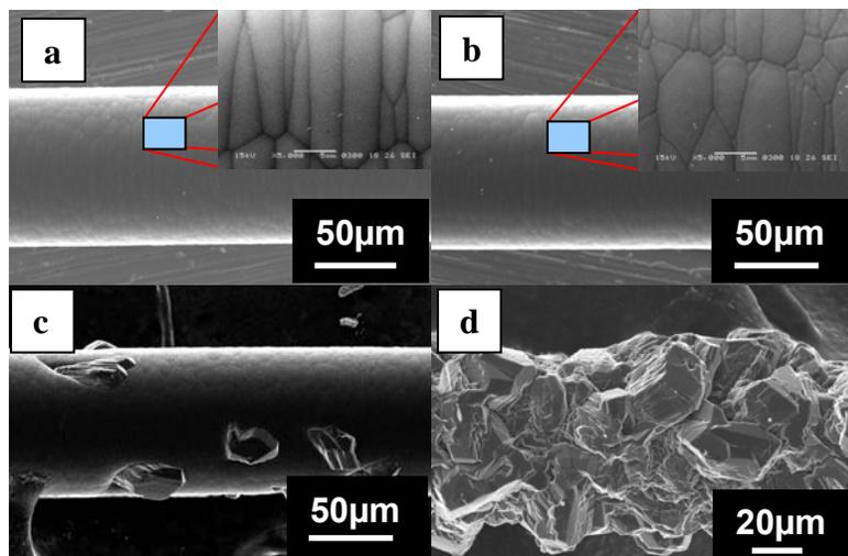
**Figure 2.** Surface morphology of boron fibers at the following carbon dopant levels in atomic percent: a) 0% b) 1.4% c) 2% and d) 3%. Insets to 2a and 2b show a 25µm wide area of the fiber surface.
