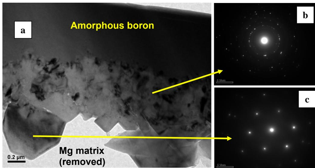
**Figure 4.** Bright-field TEM image (4a) at interface of undoped boron fiber and Mg matrix. 4b shows SAD of the finer-grained phase (SAD ring pattern consistent with MgB<sub>4</sub> or MgB<sub>12</sub>), and EDS was consistent with a phase that is more boron-rich than the MgB<sub>2</sub> phase. 4c shows SAD indexed with the [-1100] zone orientation of the MgB<sub>2</sub> hexagonal phase.
