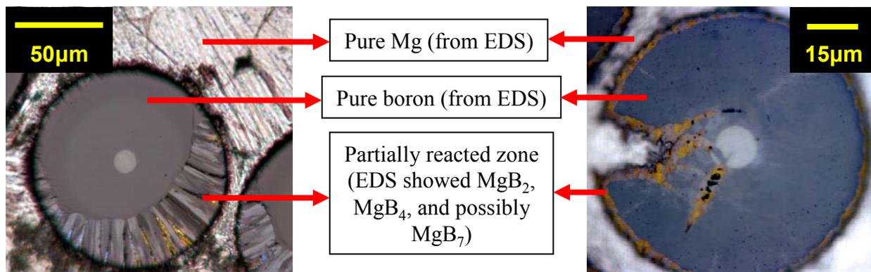
**Figure 5.** Polarized optical micrographs of composites made with undoped (left) and 0.5% C-doped (right) boron fibers. Undoped boron was heat treated at 1000°C for 15 min. C-doped boron (right) was heat treated at 1000°C for 16 hr. The Mg matrix partially reacted with the boron, although the C-doped boron fiber reacted much more slowly than the undoped fiber.
