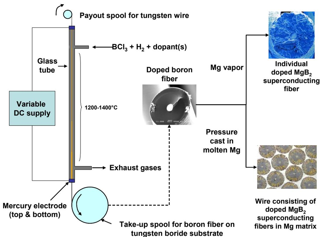
**Figure 1.** Process diagram showing CVD synthesis of boron fiber [1] and conversion to MgB<sub>2</sub> by reaction with magnesium vapor [3-7, 9] or molten Mg [8]
