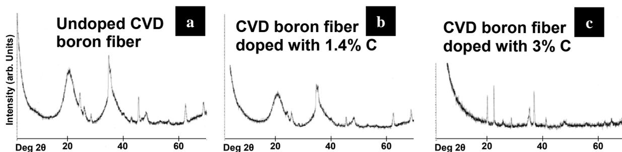
**Figure 3.** X-ray diffraction patterns of undoped and carbon-doped B fibers. Undoped boron and boron doped with 1.4% carbon consist of amorphous boron plus crystalline tungsten boride substrate material. Boron doped with 3% carbon is a well crystallized tetragonal boron phase.
