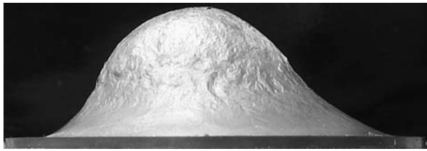
Fig. 9—Photograph of cast + HIP CP-Ti dome deformed to fracture by thermal cycling (60 cycles) under 200 kPa gas pressure (apex height: 19.7 mm).
