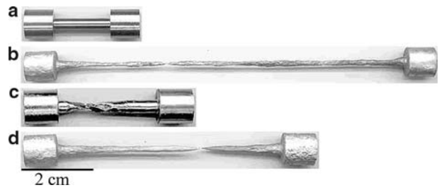
Fig. 5—Photographs of cast + HIP CP-Ti: (a) before testing, (b) after superplasticity fracture testing (511 pct elongation), and (c) after creep fracture testing (45 pct elongation). (d) Photographs of as-cast Ti-6Al-4V samples after superplasticity fracture testing (265 pct elongation).
