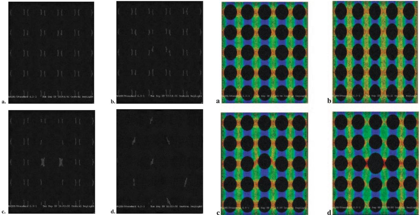
Fig. 9 Onset of local plastic deformation shown at macroscopic strain level 0.2% for several cases (a, b, c) and at macroscopic strain level 0.14% for random geometry (d). Red indicates local plasticity threshold achieved, while blue areas are in elastic regime. (a. standard, b. move in center, c. change in center; d. random combination).
