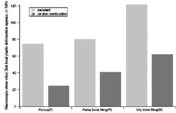
Fig. 14 Macroscopic stress when first local plastic deformation appears.
