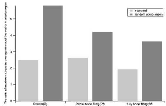
Fig. 15 A measure of the stress concentration factor: the ratio of maximum stress to average stress of the matrix under purely elastic loading (macroscopic strain applied was 0.1% in order to have no local plasticity in the matrix or bone).
