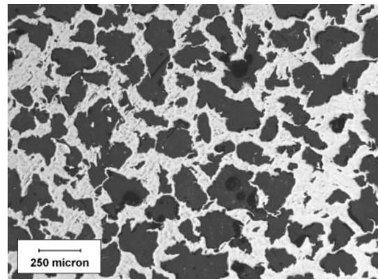
Fig. 4 Optical micrograph of Ti foam with 50% porosity, showing large, interconnected pores with ragged surfaces. Thin pore walls are also visible.
