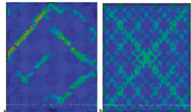
Fig. 11 Shear banding appears centered in inclusions with largest plastic deformation for fully bone filling. (a. random position, b. change in center).
