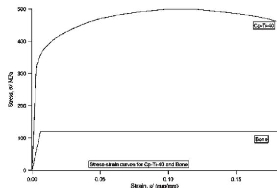
Fig. 1 Stress-strain curves for Cp Ti-40 and Bone.
