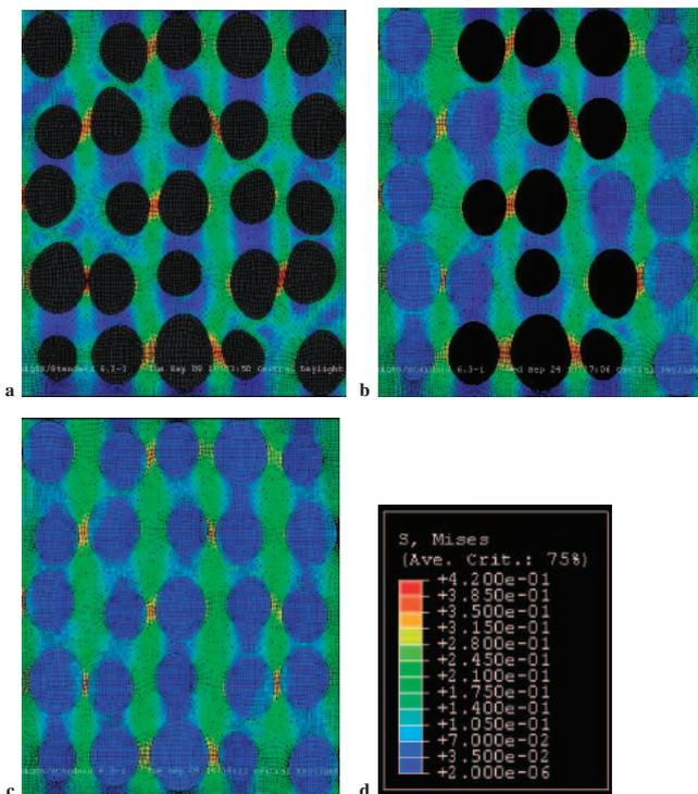
Fig. 13 Stress contour plots showing the effect of bone ingrowth on local deformation and stress fields. Macroscopic strain level is 0.2% in all cases. Note that bone ingrowth reduces local deformations and stress concentrations. The deformation shown is multiplied by the factor of 50. (a. fully porous, b. partial filled, c. fully filled, d. color scales).
