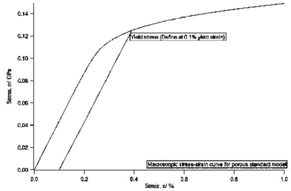
Fig. 7 Macroscopic stress-strain curve for porous standard model and definition of macroscopic yield stress.
