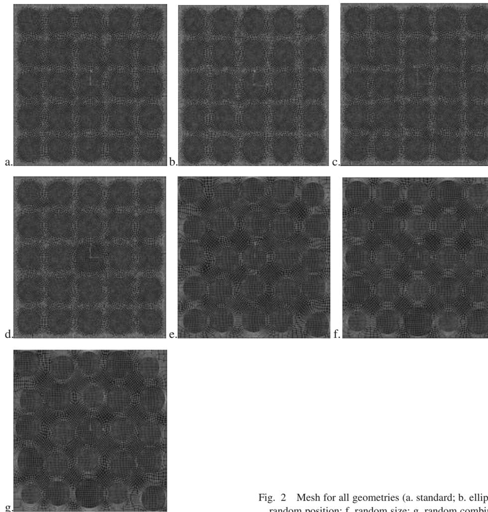
Fig. 2 Mesh for all geometries (a. standard; b. ellipse; c. move; d. size; e. random position; f. random size; g. random combination).
