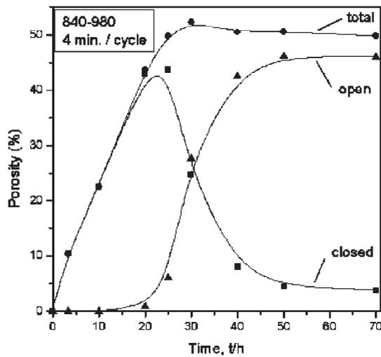
Fig. 3 Ti foam porosity (total, open and closed) as a function of time under thermal cycling conditions (4 minute cycles between 840 and 980°C).
