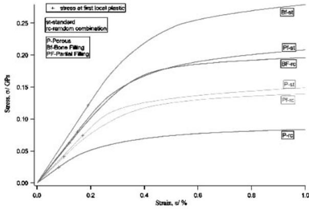
Fig. 12 Macroscopic stress-strain curve for selected models from finite element simulations. Symbols indicate the stress level at the onset of local plasticity in the matrix.
