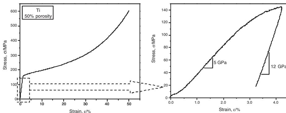
Fig. 5 Compressive stress-strain curve of foam shown in Fig. 4 with 50% porosity.
