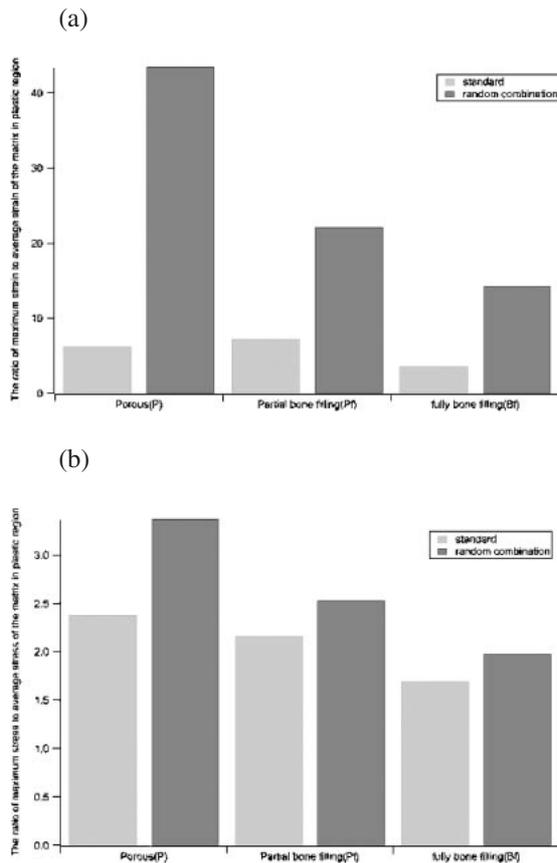
Fig. 16 (a) The ratio of maximum strain to average strain of the matrix under 0.6% applied macroscopic strain (localized plasticity prevalent). (b) The ratio of maximum stress to average stress of the matrix under 0.6% applied macroscopic strain (localized plasticity prevalent).
