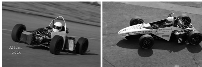
Fig. 10. Crash protector in a model racing car built by students at the University of Technology of Stralsund, Germany; a) view of car with the front encasement taken off, b) full view (Courtesy of Sönke Reinhardt).
