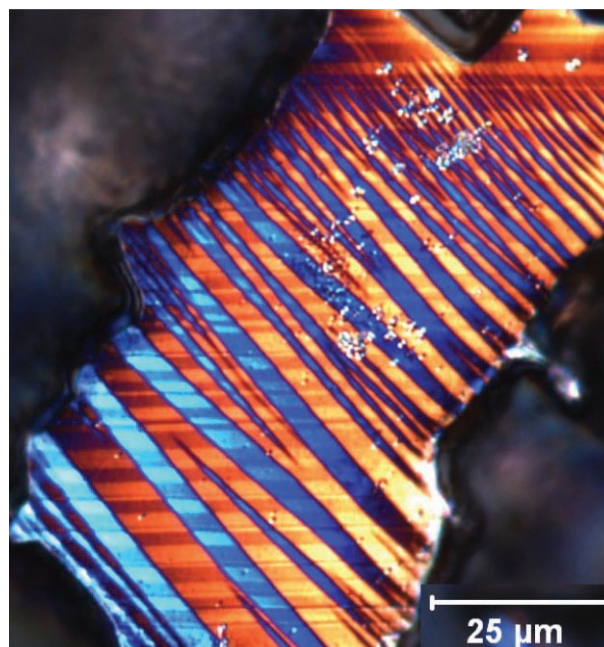
Figure 10. Cross-section of strut in Ni-Mn-Ga foam with twins spanning the width of the strut within a single bamboo grain. Reprinted with permission from [19]. Copyright 2009, Nature Publishing Group.
