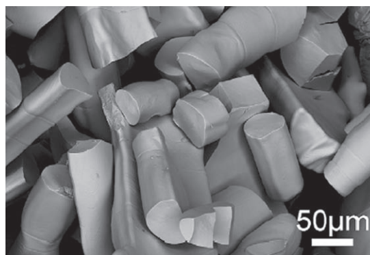
Figure 4. Short Ni-Mn-Ga fibers created by mortar grinding of longer fibers, composed of single or few grains spanning the fiber width. Reprinted with permission from [91]. Copyright 2007, Elsevier.
