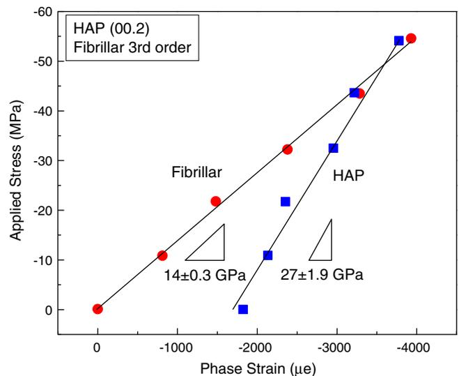
Fig. 5. Plot of applied stress vs. longitudinal elastic strain for the fibril (SAXS) and HAP (WAXS, HAP (00.2) reflection) for a point located 2.5 mm from the buccal edge and 2 mm from the lingual edge in a fresh, uncycled dentin sample taken from the bottom of a fourth incisor on the right side of the jaw from the point of view of the animal.
