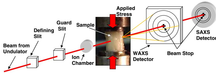
Fig. 1. Schematic of the experimental diffraction setup showing a photograph of the bovine dentin sample. The height of the sample is 7.5 mm.
