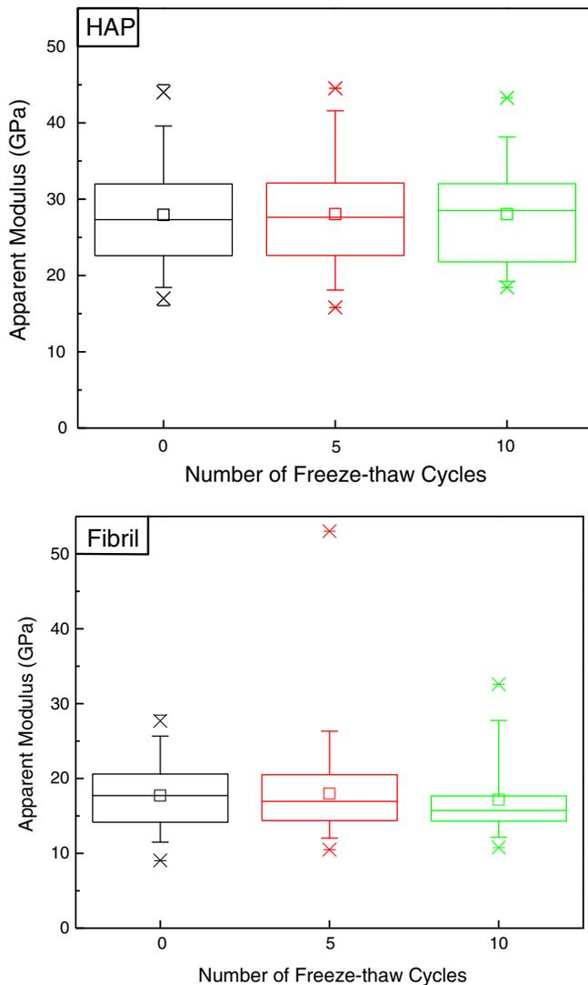
**Fig. 6.** Box plots showing the mean ( $\square$ ), maximum and minimum values ( $-$ ), as well as the 99th and 1st ( $x$ ), 95th and 5th (whiskers), and 75th, 50th, and 25th percentiles (box) for HAP and the fibril apparent modulus for the entire populations of samples uncycled (12 specimens: O, A, B, C), after 5 freeze–thaw cycles (6 specimens: A, B), and after 10 freeze–thaw cycles (3 specimens: A).
