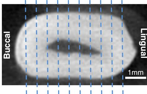
Fig. 2. Lab micro-computed tomography image of a sample from group O taken from the bottom of a left third incisor. The dotted lines represent the path of the beam during measurement.
