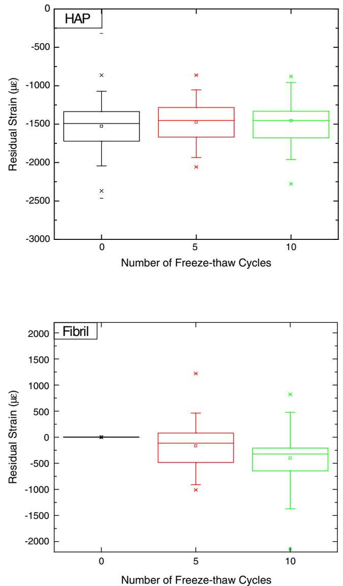
**Fig. 7.** Box plots showing the mean ( $\square$ ), maximum and minimum values ( $-$ ), as well as the 99th and 1st ( $x$ ), 95th and 5th (whiskers), and 75th, 50th, and 25th percentiles (box) for HAP and fibril residual strain for the entire populations of samples uncycled (12 specimens: O, A, B, C), after 5 freeze–thaw cycles (6 specimens: A, B), and after 10 freeze–thaw cycles (3 specimens: A).
