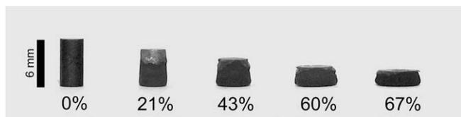
Fig. 2. Photographs of a specimen of sample B deformed to an engineering compressive strain of 67% (true strain of  $-1.1$ ) in four stages at  $1000^\circ\text{C}$  without any cracking. Initial and final  $\text{MgB}_2$  specimen heights are 6.0 and 2.0 mm. Initial strain rate for each stage was maintained at  $4 \times 10^{-5} \text{ s}^{-1}$ .
