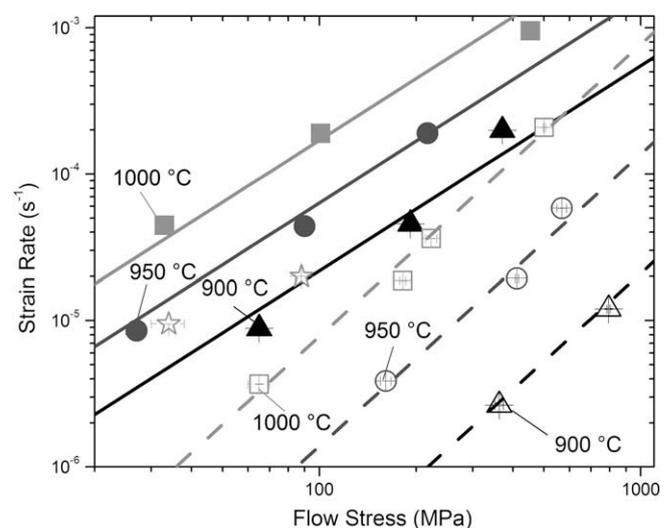
Fig. 6. Double-logarithm plot of compressive strain rate vs. flow stress for 900, 950 and 1000 °C, with best-fit lines determined from Eq. (1) for specimens A (data from Fig. 4 as filled symbols, best-fit lines are continuous) and B (data from Fig. 5 as open symbols, best-fit lines are dashed). The two tensile flow tests at 1000 °C are shown with open star symbols. Error bars correspond to one standard deviation.
