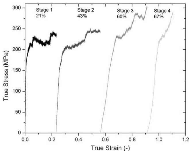
Fig. 3. Compressive stress–strain curves for a specimen of sample B deformed in four stages to 67% compression (true strain  $-1.1$ ) at a strain rate of  $4 \times 10^{-5} \text{ s}^{-1}$ . Photographs of the specimen at the end of each stage are shown in Fig. 2.
