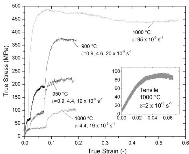
Fig. 4. Compressive stress–strain curves for specimens of sample A tested at 900, 950 and  $1000^\circ\text{C}$  at constant strain rates varying between 0.9 and  $95 \times 10^{-5} \text{ s}^{-1}$ . Inset shows a tensile stress–strain curve of a specimen of sample B.
