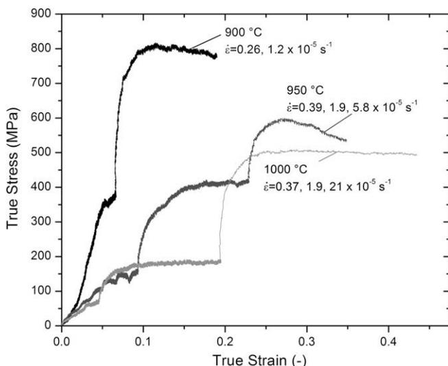
Fig. 5. Compressive stress–strain curves for specimens of sample B tested at 900, 950 and 1000 °C at constant strain rates from 0.26 to  $21 \times 10^{-5} \text{ s}^{-1}$ .
