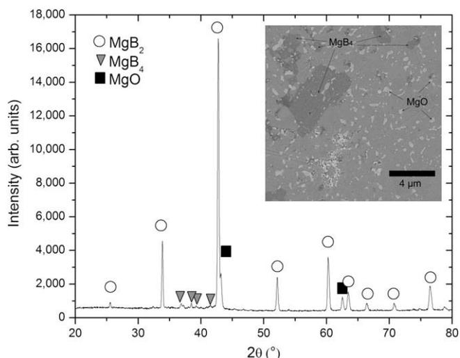
Fig. 1. XRD pattern for as-densified specimen A, identifying  $\text{MgB}_2$  as the main phase and  $\text{MgB}_4$  and  $\text{MgO}$  as minor phases. These phases are also visible with backscattered scanning electron microscopy (inset).
