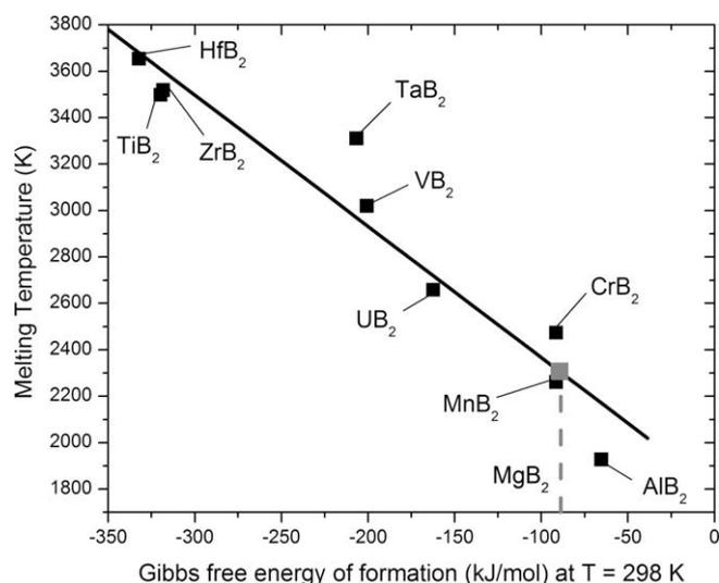
Fig. 7. Plot of melting point vs. Gibbs free energy of formation for nine isostructural  $\text{AlB}_2$ -type diborides (data from Ref. [50]). The best-fit line predicts a melting point of  $2307 \text{ K}$  for  $\text{MgB}_2$ , based on its free energy of formation of  $-89.5 \text{ kJ mol}^{-1}$  [50].
