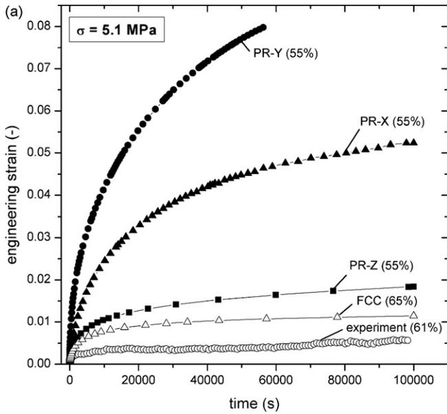
Fig. 4. Creep strain as a function of time obtained by FEM for FCC sphere arrangement ( $f = 65%$ ) and PR sphere arrangement ( $f = 55%$ ) at  $500^\circ\text{C}$  for a compressive stress of 5.1 MPa. Curves for PR arrangement are shown for deformation along the three main axes. For comparison, the corresponding experimental foam creep curve is also plotted for a foam with  $f = 61%$ .
