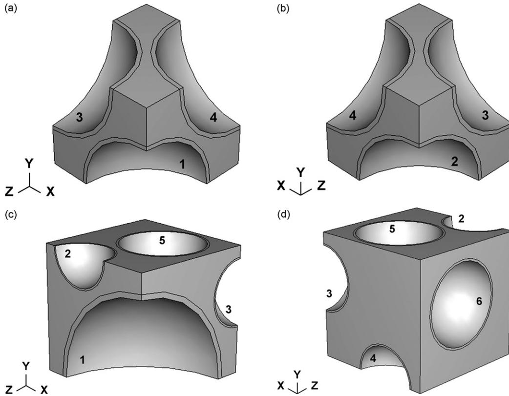
Fig. 3. Unit cells used for FEM: (a) face cubic centered (FCC) sphere arrangement with sphere volume fraction  $f=65\%$ ; (b) as (a) but rotated  $180^\circ$  around the  $Y$  axis; (c) pseudo-random (PR) sphere arrangement with  $f=55\%$ ; and (d) as (c) but rotated  $180^\circ$  around the  $Y$  axis. Uniaxial compressive stress is applied along one of the main axes.
