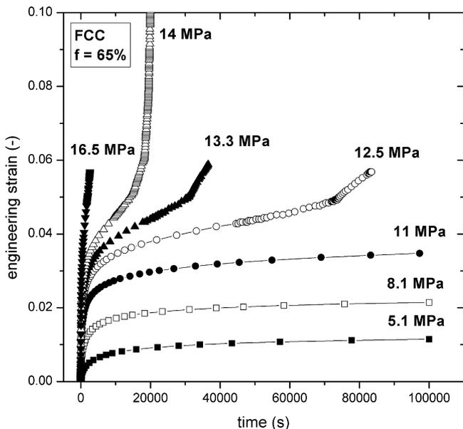
Fig. 5. Creep strain as a function of time obtained by FEM for foams with FCC sphere arrangement ( $f = 65%$ ) for various compressive stresses at  $500^\circ\text{C}$ .
