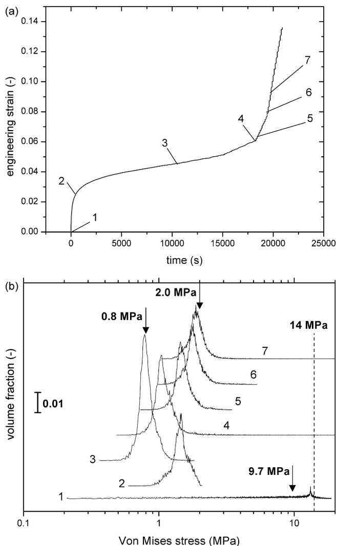
Fig. 7. (a) Creep strain as a function of time as calculated from FEM for FCC sphere arrangement ( $f = 65\%$ ) deformed at  $500\text{ }^{\circ}\text{C}$  under  $14\text{ MPa}$  stress; (b) corresponding von Mises stress distribution in the matrix, calculated at seven creep strains labeled in (a). The volume average von Mises stress is indicated for histograms 1, 3 and 7. The applied stress is marked with a vertical dotted line.
