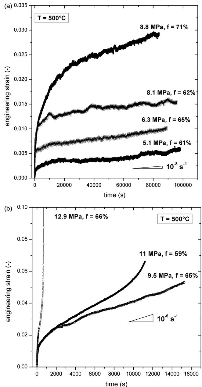
Fig. 2. Creep strain as a function of time measured for foams (with volume fractions  $f=59$ –71%, indicated next to each curve) deformed at 500 °C for compressive stresses: (a) below 9 MPa and (b) above 9 MPa.
