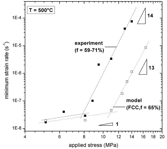
Fig. 6. Minimum strain rate as a function of applied compressive stress as determined by FEM for FCC sphere arrangement ( $f = 65%$ ), and as measured experimentally on syntactic foams ( $f = 59-71%$ ).
