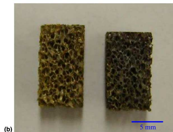
Fig. 7. (a) Typical creep curve for Ni–9.1Al foam ( T = 725 °C, \sigma = 0.21 MPa). (b) Specimens before and after creep test showing a macroscopically uniform deformation.
