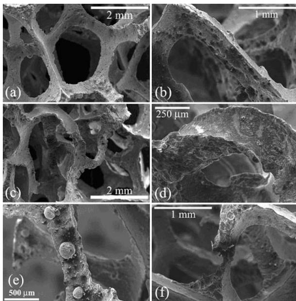
Fig. 3. Scanning electron micrographs illustrating common structures and defects in graded aluminum foam. (a) pore structure in the low-density region; (b) a typical nearly-straight strut in the low-density region; (c) pore structure in the high-density region; (d) a heavily deformed strut in the high-density region; (e) example of replicated bubbles from imperfect investment settling; (f) example of major strut defect.
