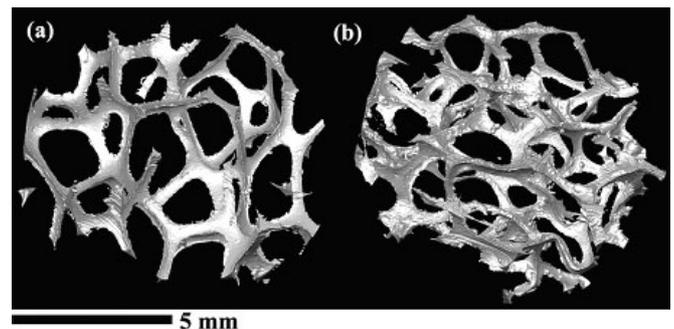
Fig. 4. Tomographic renderings of selected volumes from the graded sample in Figures 2 and 3, taken near: (a) the low-density face; and (b) the high-density face. The scale bar is approximate.
