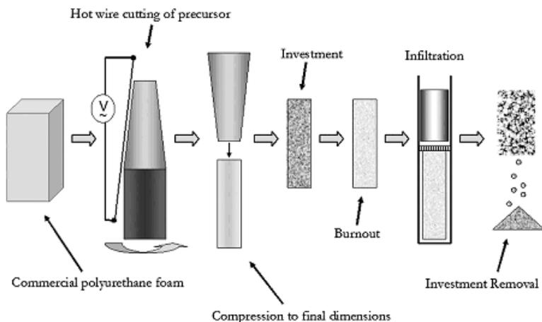
Fig. 1. Schematic illustration of the replication method developed for production of continuously-graded metallic foams.
