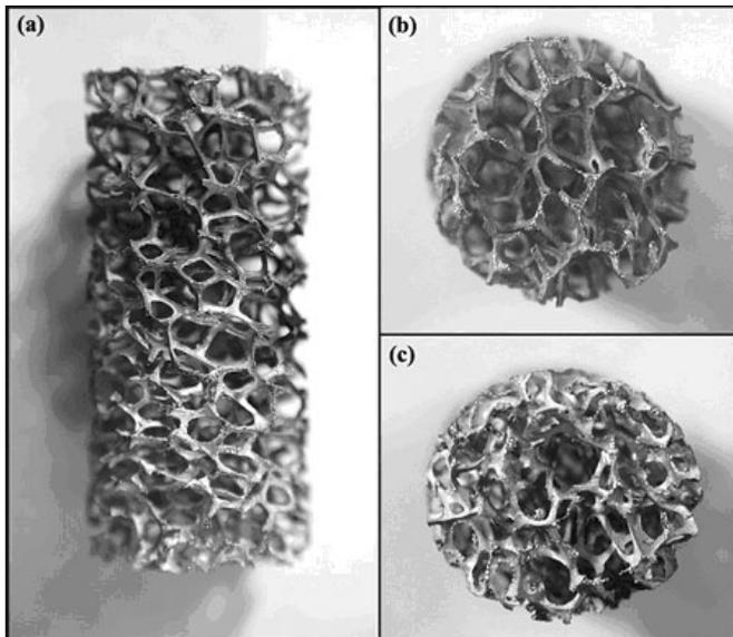
Fig. 2. Photographs of a graded aluminum foam sample processed by the method illustrated in Figure 1. (a) side view, with the low-density face at the top of the panel and the high-density face at the bottom; (b) end view of the low-density face; (c) end view of the high-density face. The diameter of the foam is ca. 14 mm.
