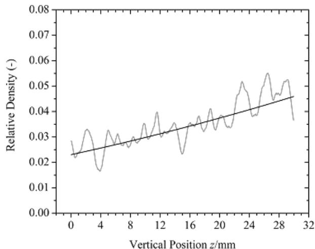
Fig. 6. Relative density profile calculated from the radiographic data in Figure 5(b). Also shown for comparison is the predicted relative density profile estimated from precursor dimensions.
