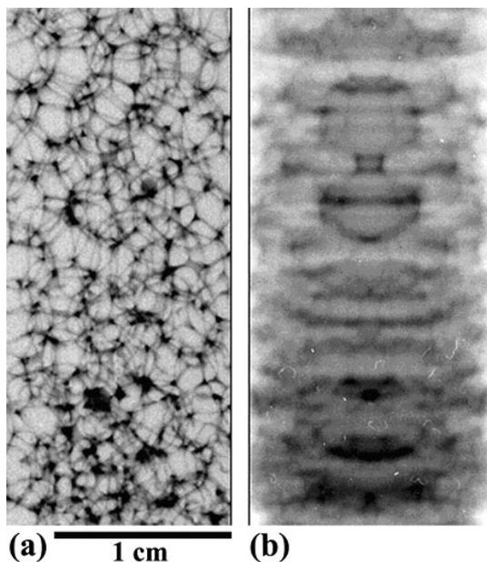
Fig. 5. Radiographic images of the graded foam sample of Figures 2–4, with the low-density face at the top of the panel and the high-density face at the bottom. (a) radiograph of the stationary sample; (b) radiograph of the rotating sample. Radiographs have been contrast-enhanced for better visualization.
