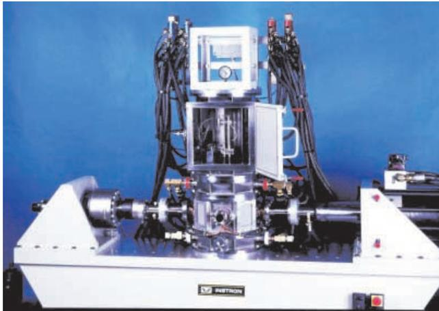
Fig. 6. Load frame with furnace mounted
