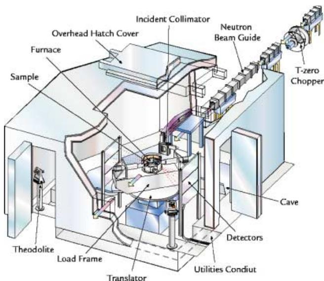
Fig. 3. Cutaway Schematic of cave
